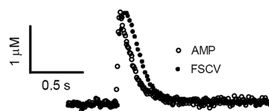
Figure 1. Stimulated dopamine release monitored with fast-scan cyclic voltammetry repeated at 60 Hz and amperometry. Both measurements were in the presence of 500 \mu\text{M} ascorbate. A time delay due to adsorption can be seen in the fast-scan cyclic voltammetric response indicated by a longer time to reach a maximum and a slower decay to baseline. The adsorptive delay with cyclic voltammetry was accounted for using the convolute-and-compare method to obtain rate constants. Reprinted with permission from ref 11. Copyright 2012 American Chemical Society.
